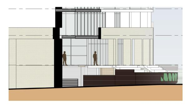
b) The side elevations presented bland blank walls to the east and west. Articulation to break up those facades is needed through architectural features and/or a mix of materials.
